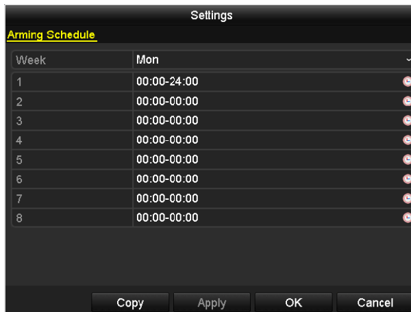
Figure 8-17 Set Arming Schedule of Alarm Output
