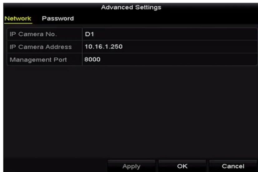
Figure 2-36 Network Configuration of the Camera
